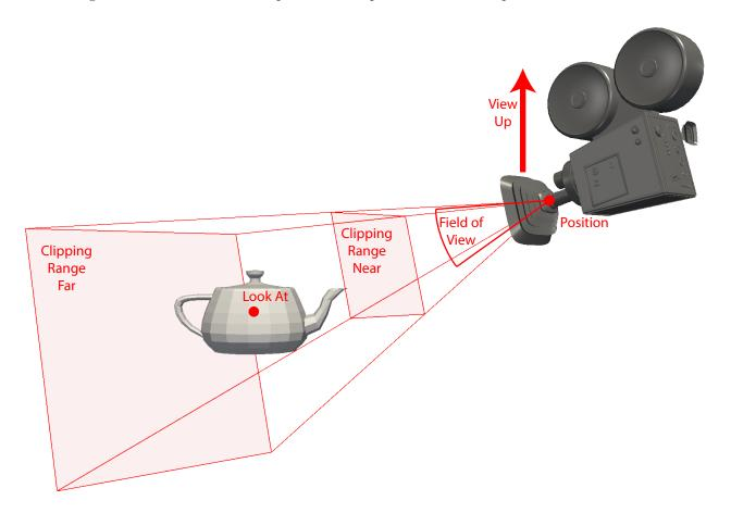
Figure 5.4: The position and orientation parameters for a Camera.
