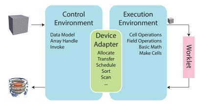
Figure 6.1: Diagram of the VTK-m framework.
