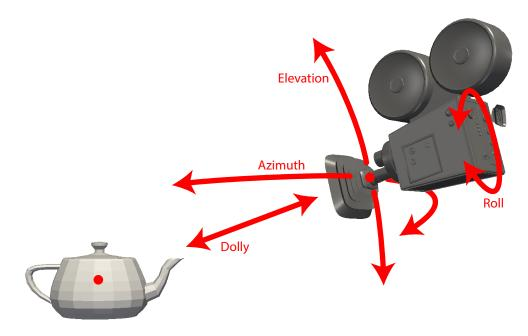
Figure 5.5: Camera movement functions relative to position and orientation.
