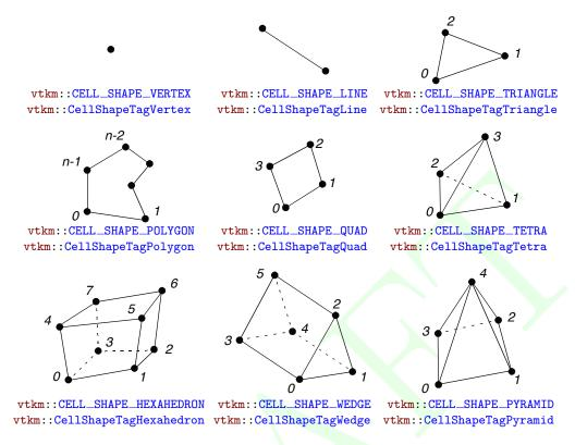
Figure 17.1: Basic Cell Shapes
