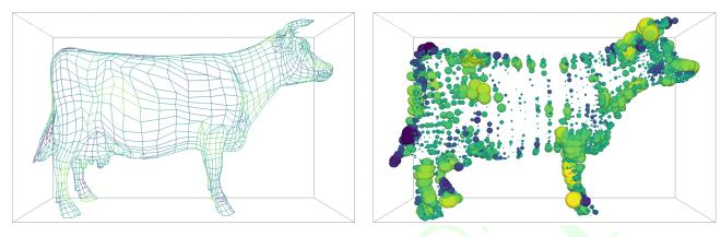
Figure 5.2: Examples of alternate rendering modes using different mappers. The left image is rendered with MapperWireframer. The right image is rendered with MapperPoint.
