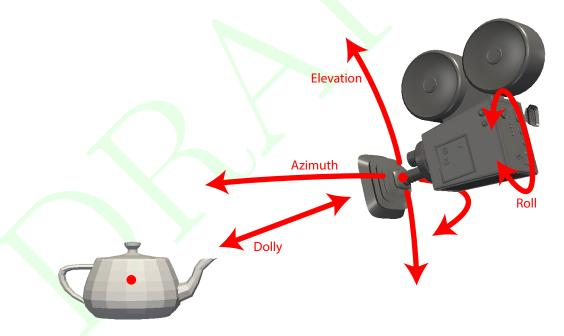
Figure 5.5: Camera movement functions relative to position and orientation.
