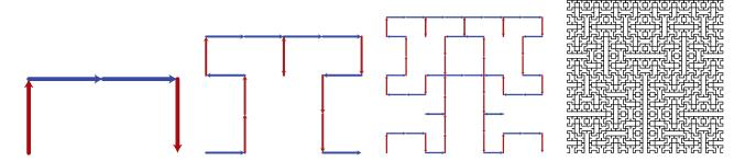
Figure 41.9: The first, second, third, and sixth iterations, respectively, of the Hilbert curve fractal.
