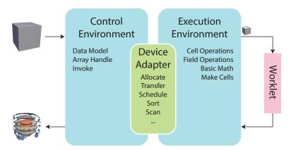
Figure 15.1: Diagram of the VTK-m framework.
