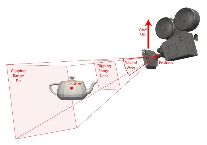
Figure 10.4: The position and orientation parameters for a Camera.
