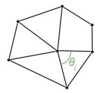
Figure 28.1: The angles incident around a point in a mesh.
