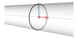
Figure 14.3: Visual Representation of an Implicit Cylinder. The red dot represents the center value, and the red arrow represents the vector that points in the direction of the axis. The radius is the length of any line (like the blue one shown here) that extends perpendicular from the axis to the surface.
