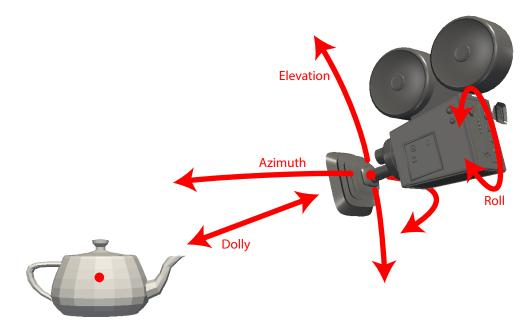
Figure 10.5: Camera movement functions relative to position and orientation.
