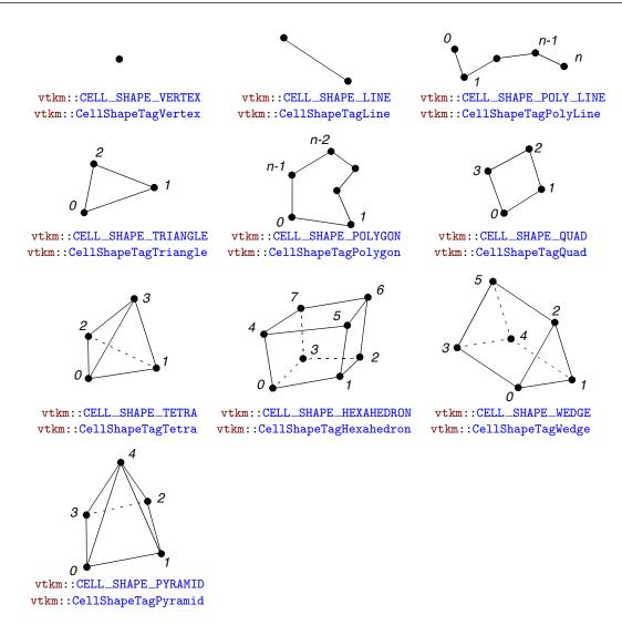
Figure 7.5: Basic Cell Shapes in a CellSetExplicit.
