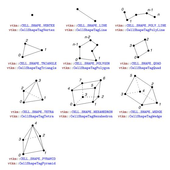
Figure 25.1: Basic Cell Shapes
