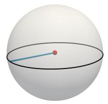
Figure 14.2: Visual Representation of an Implicit Sphere. The red dot represents the center of the sphere. The radius is the length of any line (like the blue one shown here) that extends from the center in any direction to the surface.
