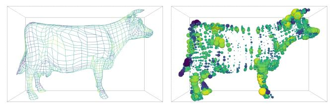
Figure 10.2: Examples of alternate rendering modes using different mappers. The left image is rendered with MapperWireframer. The right image is rendered with MapperPoint.
