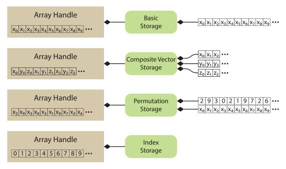
Figure 36.1: Array handles, storage objects, and the underlying data source.
